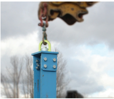
Step 1. With Panel Puller removed from packaging, connect machine to top of puller and move toward working area
