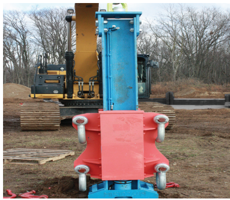
Step 2. Position Panel Puller so that when it is laid on the ground the hose connections are facing up.
