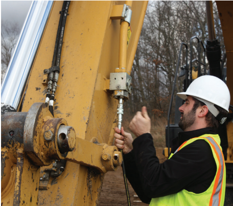
Step 4. Using the proper quick connect (not supplied) for a power pack or machines aux. hydraulic system, connect hoses. Verify secure connection.
