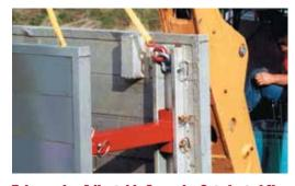
Telescoping Adjustable Spreader Sets (set of 4)
