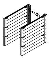
4. Install factory approved lift eyes, then install the remaining panels to desired height ensuring that all matching holes have a pin and keeper.
