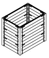
6. The 4th corner post can then be slid into place, A prybar may be needed to align post with holes. All matching holes require a pin and keeper.
