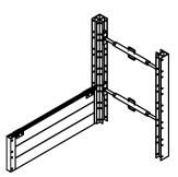
2. Set back spreaders at required spacing (refer to tabulated data) and 2nd corner post. Install pins and keepers in all matching holes.
