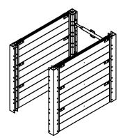
Add 3rd and 4th corner post ensuring that all matching holes have a pin and keeper. Install remaining lift eyes.
