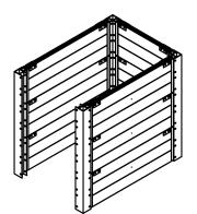
Add opposite panels to desired height. Add 4th corner post. Ensuring that all matching holes have a pin and keeper. Install remaining lift eyes.  Install factory approved lift eyes, then install 2nd and 3rd corner post. Ensuring that all matching holes have a pin and keeper.
