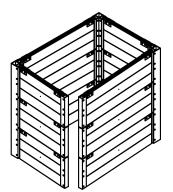
5. Add opposite panels to desired height. All matching holes require a pin and keeper. Install remaining lift eyes.
