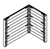
4. Install factory approved lift eyes, then install 2nd and 3rd corner post. Ensuring that all matching holes have a pin and keeper.
