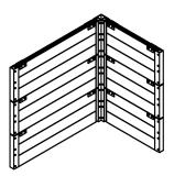
3. Stack panels to desired height before adding 2nd corner post.
