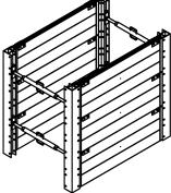
Install spreaders at required locations (refer to tabulated data). All matching holes require a pin and keeper.
