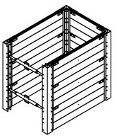
6. Install spreaders at required locations (refer to tabulated data). All matching holes require a pin and keeper.
